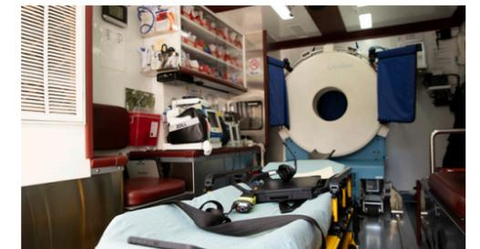
The unit is a specially modified ambulance with a CT scanner onboard
