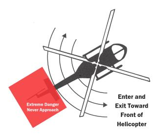
When working around helicopters, never approach from the rear. Always approach and depart the aircraft towards the front or side so you can see the pilot, and he can see you. Only approach the helicopter under the supervision of a flight crew member. When approaching the helicopter, remember to keep low to avoid main rotor, because winds can cause the rotor to flex down.
